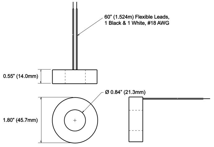
Figure 8 – M000530 100A Current Transducer
