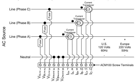
Figure 5 – Three-Phase Wye Connection Diagram
