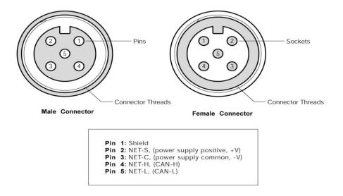
Figure 2 – NMEA 2000<sup>®</sup> Connector Face Views
