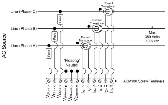
Figure 6 – Three-Phase Delta Connection Diagram
