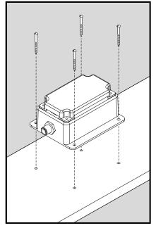
Figure 1 – Mounting the ACM100
