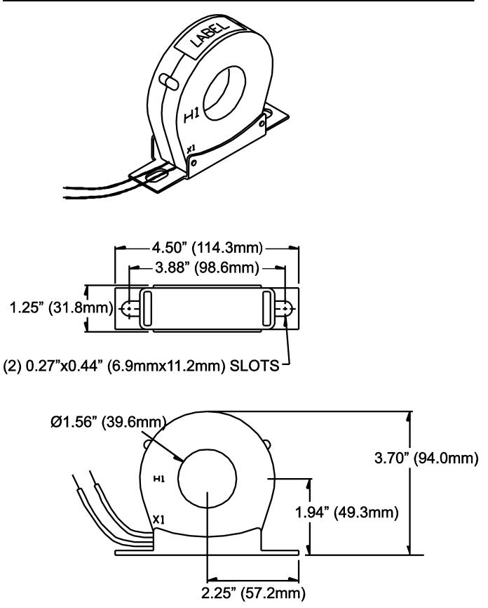
Figure 9 – M000612 400A Current Transducer
