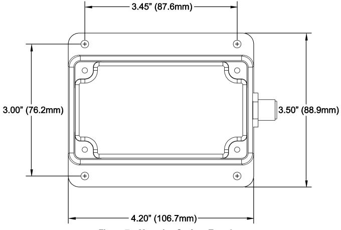
Figure 7 – Mounting Surface Template
