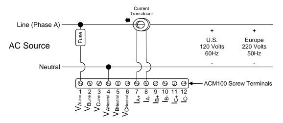
Figure 3 – Single-Phase (Single Line) Connection Diagram
