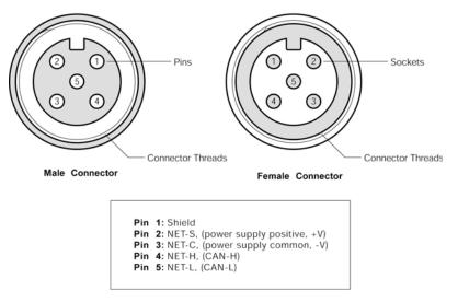
Figure 2 – NMEA 2000<sup>®</sup> Connector Face Views
