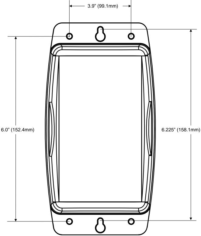
Figure 4 – Mounting Template
