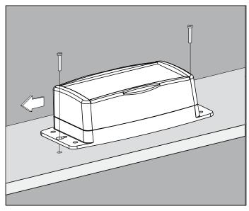
Figure 1 – Mounting the SMS100
